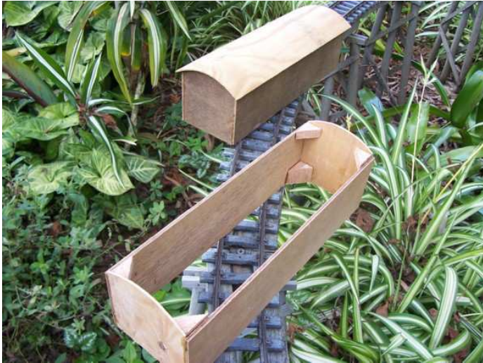
Roof arcs are formed from wetted 2mm plywood.
