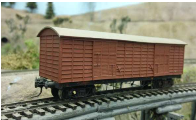
The CLF Class had two doors each side. It has Louvered cladding all around.
