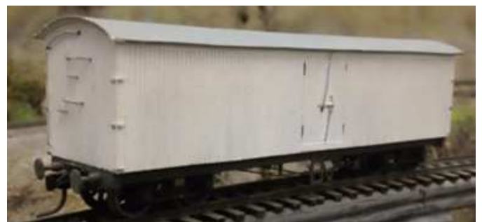
Some had Louvre end walls, others had diagonal side cladding.
