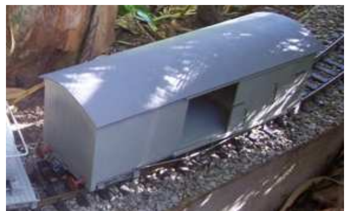
Completed C Class bogie 'Box' car, scratchbuilt in wood, with working slide doors.
